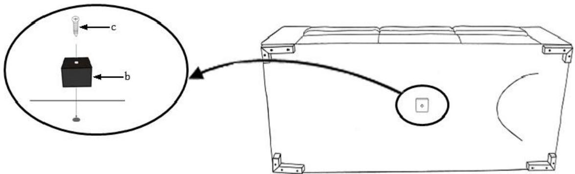
STEP 5: Cover the holes of L shaped legs (a) and middle leg (b) with plastic caps (d)
