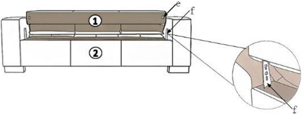
STEP 2: Push the back frame (1) vertically straight down to seat frame (2), until it is securely "locked" in place.
