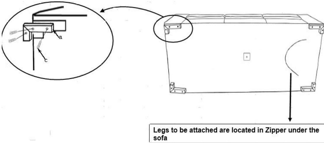
STEP 4: Fasten the middle leg (b) with screws (c)
